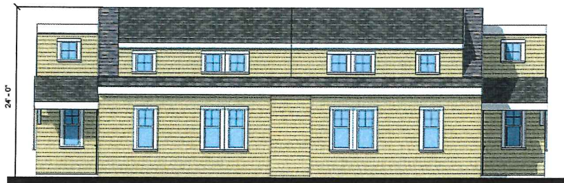
22 TYPICAL 2 STORY ELEVATION - BACK Scale : 1/8" = 1'-0"
