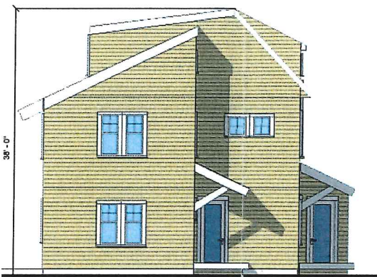
11 TYPICAL 3 STORY ELEVATION - B - SIDE A Scale : 1/8" = 1'-0"
