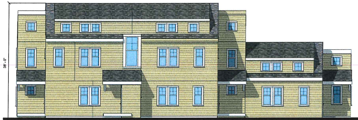
20 TYPICAL 3 STORY ELEVATION - BACK Scale : 1/8" = 1'-0"
