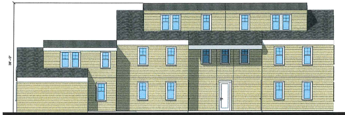
21 TYPICAL 3 STORY ELEVATION - FRONT Scale : 1/8" = 1'-0"
